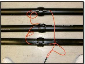
You can ensure that you have connected the fittings correctly and that the welds are successful by checking that all of the connected fittings get warm and that all of the indicator pins are exposed at the end of the welding time.
