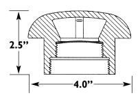
The Emco Wheaton A0785 Downward Mushroom Vent is designed for downward venting of storage tanks. The 30 mesh stainless steel screen can be easily removed for cleaning. The A0785 threads onto either 1.5 or 2.0 inch vent lines. Clear coated aluminum for corrosion-free service.
